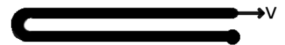
Figure 2: Carpet: Lower end fixed, upper end being pulled at constant velocity v
